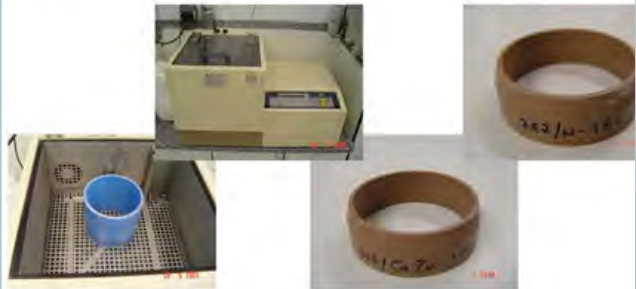
Assessment of PVC degree of gelation – Dichloromethane (EN 580) or acetone (ASTM D2152) immersion test
