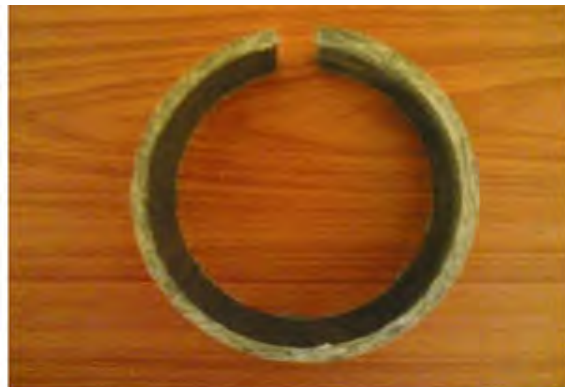
Figure 2. The ring cuts off from PVC pipe.
